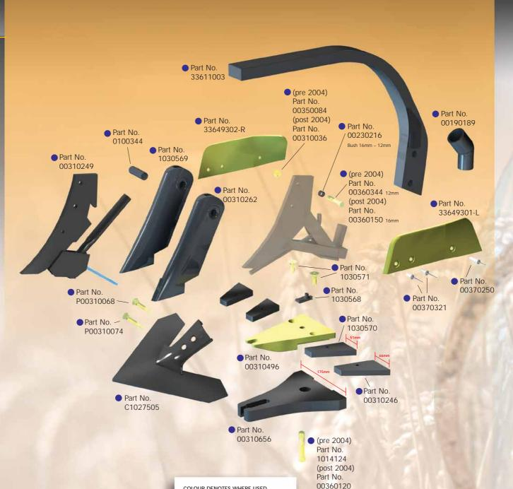
All parts shown are right handed. When parts are available right or left handed this is indicated with 'R' or 'L' after part No.
